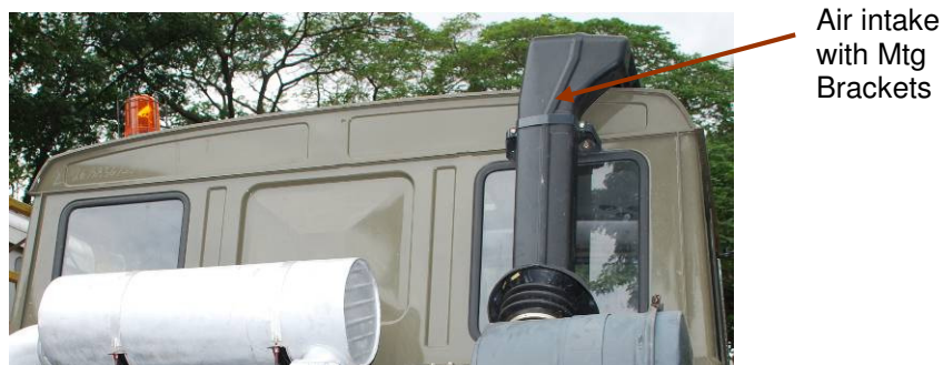
Fig 16: Air intake with mounting Brackets
