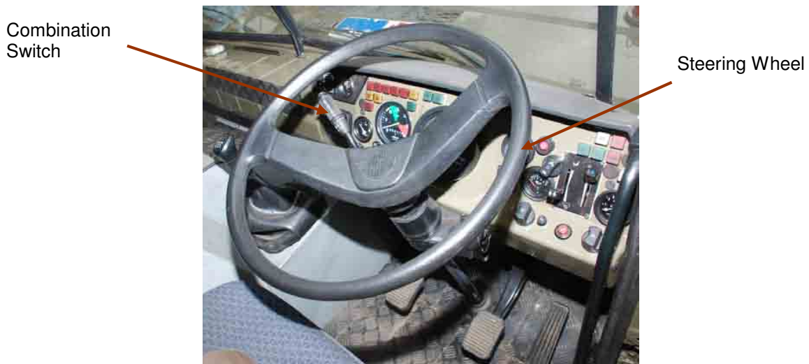
Fig 11: Steering Wheel and Single Lever combination switches
