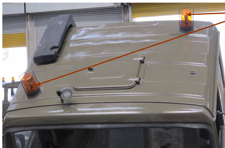
Fig 13: Beacon lamps with metal guards fitted on cabin roof
