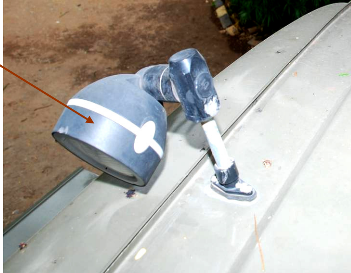
Fig 12: Search light fitted on cabin roof
