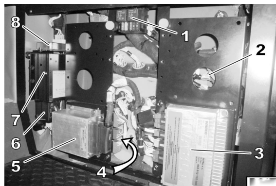
Figure 37 Central Electric Panel
