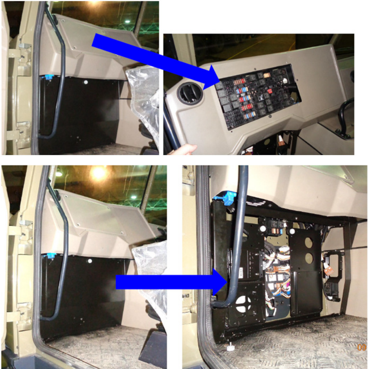
Figure 35 Overview of fuses, relays and diodes in the fuses box
