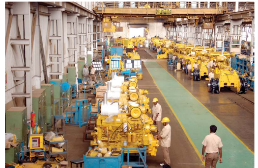
Dozer Assembly Line at BEML KGF Plant
