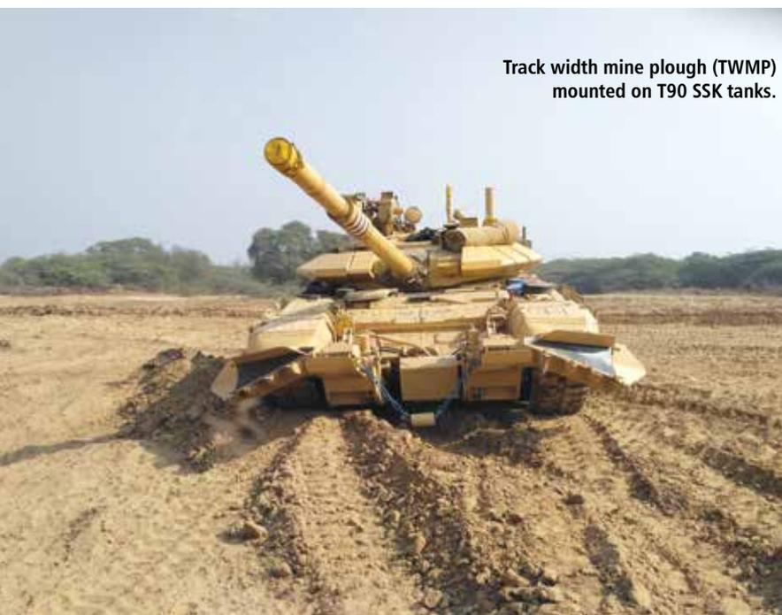
**Track width mine plough (TWMP) mounted on T90 SSK tanks.**
