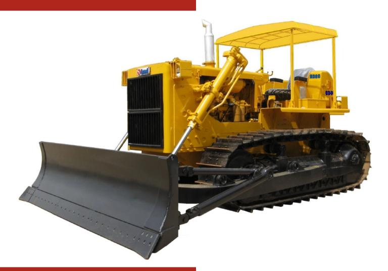
Flywheel horsepower (net) : 134 kW (180 hp) @ 1850 rpm
