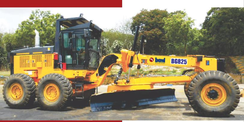
Flywheel power (net) : 209 kW (280 hp) @ 2100 rpm
