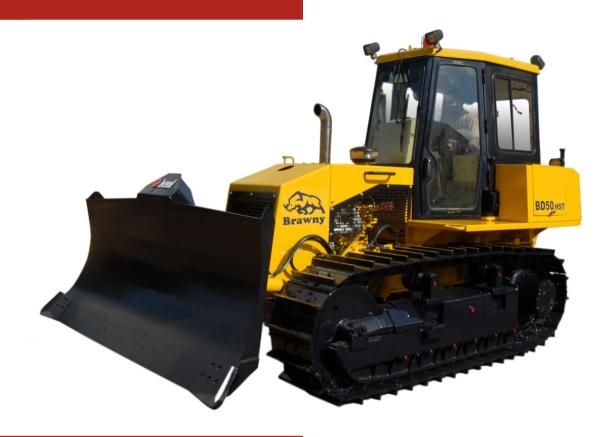
Flywheel horsepower : 75kW (100 hp) @ 2200 rpm
