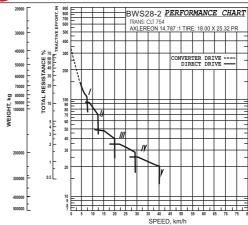
**How to use this chart:** Draw a straight line from gross vehicle mass to percent of total resistance (total resistance = grade resistance + rolling resistance) and extend the same line upto tractive effort. From this point draw horizontally to the curve with the highest obtainable gear, then vertically down to obtain maximum speed.
