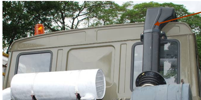
Fig 16: Air intake with mounting Brackets
