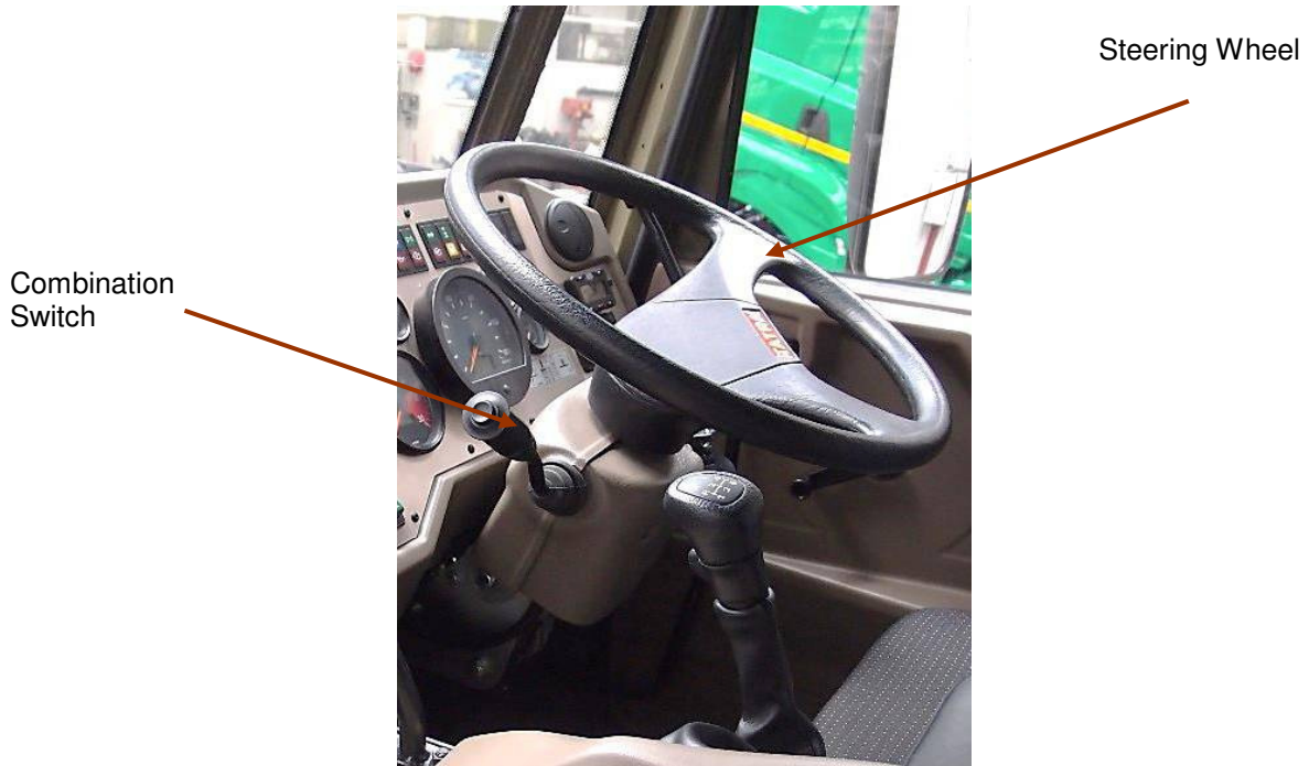
Fig 11: Steering Wheel and Single Lever combination switches
