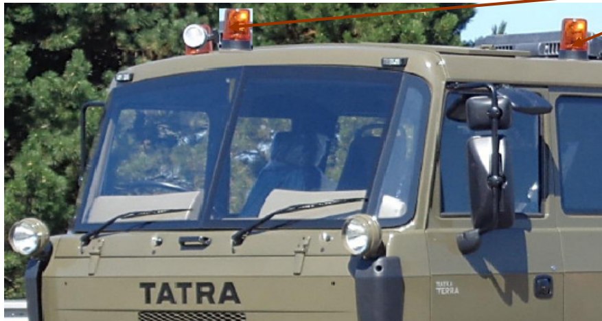
Fig 13: Beacon lamps with metal guards fitted on cabin roof
