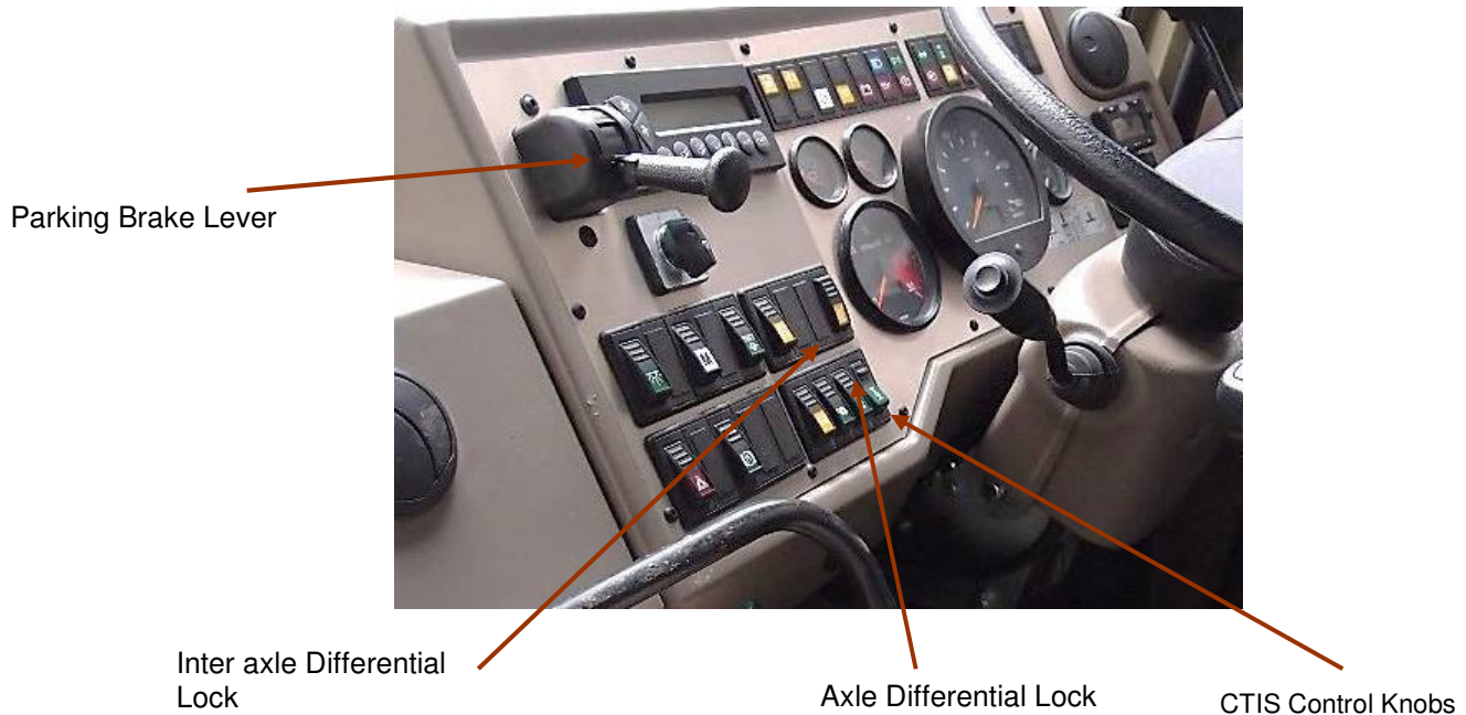
Fig 5: Parking brake and controls for drive selection
